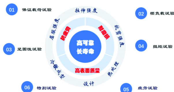
图1 紧固件性能相关性分析图 Fig. 1 Correlation analysis chart of fastener performance
